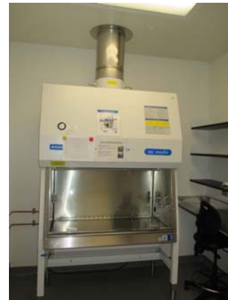
256060e 5/11/2021 Vented bio-safety cabinet Room 4210C
